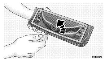
$3. \ \mbox{Pull}$  bulb straight from socket to remove.
